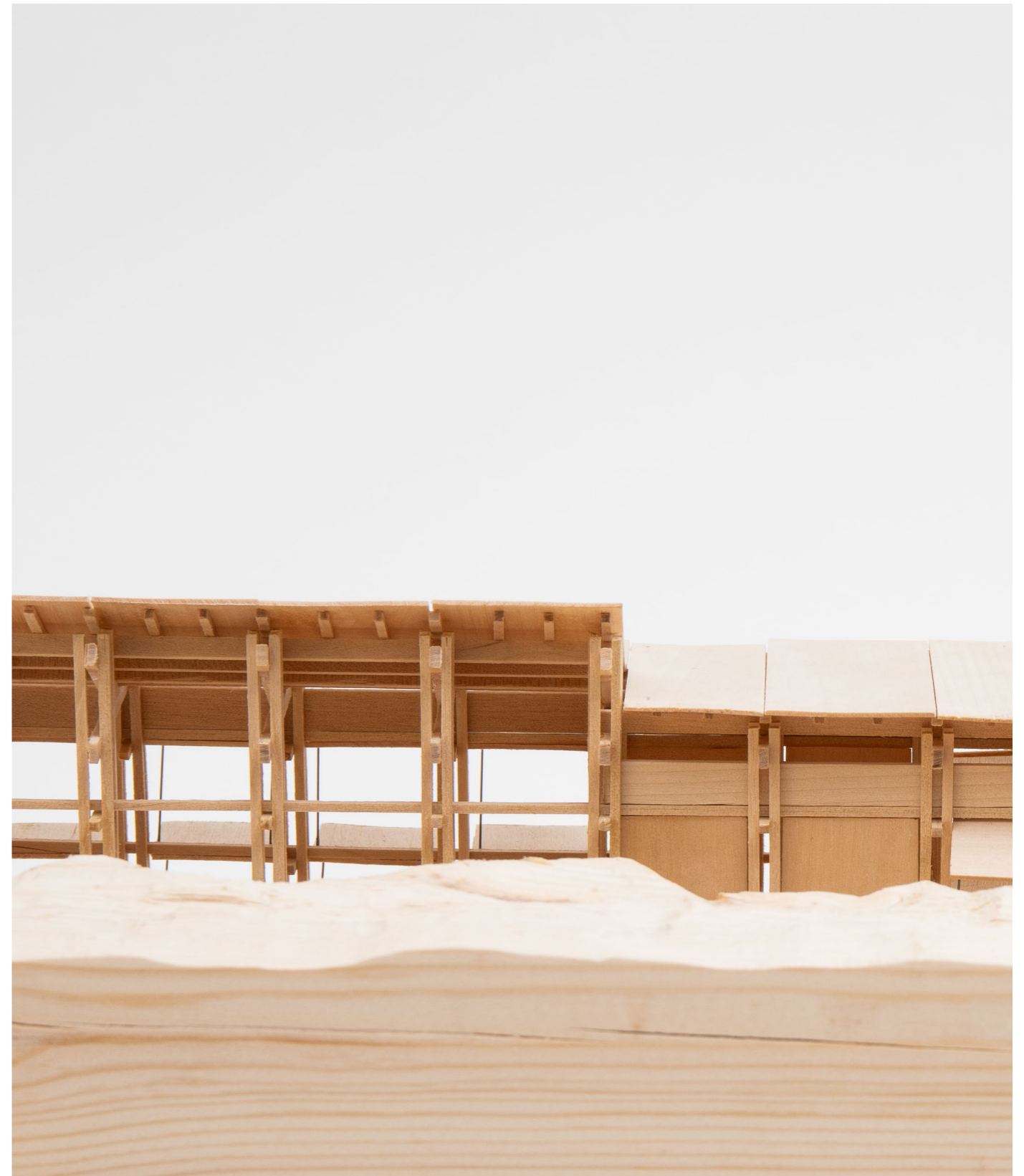
Construction model 1:50. Roof tilted up towards the the stone wall. Two additional lifts are made along the path, towards the neighborhood and the forest
