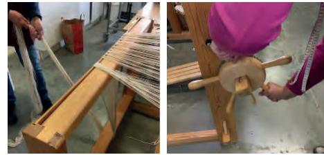
Figure 2 One is holding the warp (to the left); The other is winding the warp (to the right)
