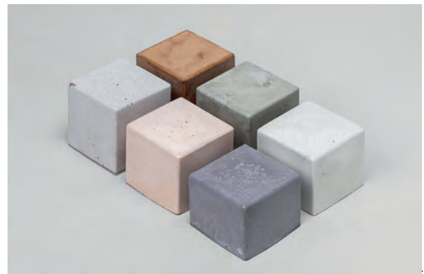
Figure 2: Selected geopolymers test cubes. Clockwise from the back: calcined Finnish clay, raw Finnish clay, chamotte, volcanic rock, feldspar, and porcelain waste. Photo: Johannes Kaarakainen, 2022.
