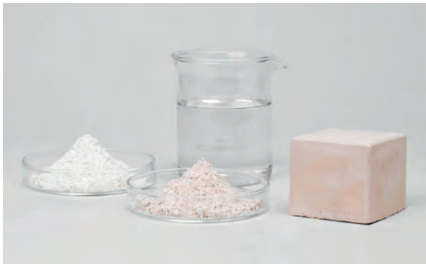
Figure 8: From left: metakaolin, potassium feldspar and sodium silicate. The cube on the right is a finished sample made with potassium feldspar as the filler component. Photo: Johannes Kaarakainen, 2022.
