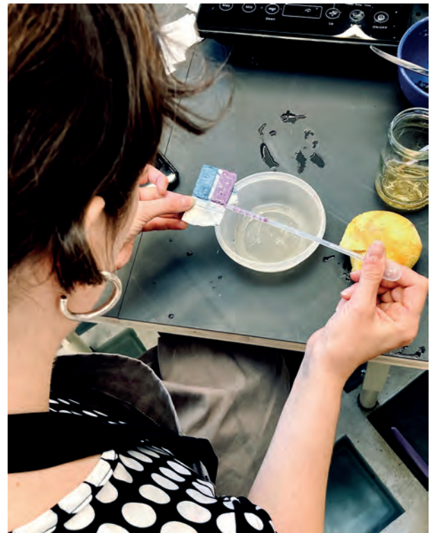
Fig.8: P9 changing the color of red cabbage by adding citric acid on one half of her DSSC
