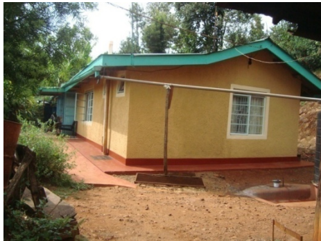
Fig. 5.64 Mr. Nyaga's Main House. (Source: Author, 2009) The walls are mud block with a rough spray plaster on the outside and painted a cinnamon color.
