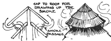
Fig. 4.20 Proposed roof vents. (Source: Koeune, 1961)
