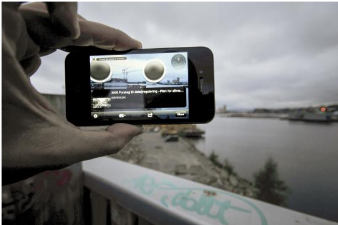
Figure 1: PlanAR—Mapping the archive on the city through augmented reality. Case title and a sampled case file illustration emerges when a marker is centred, providing a direct link to the case file. The size of the markers reflects distance.
