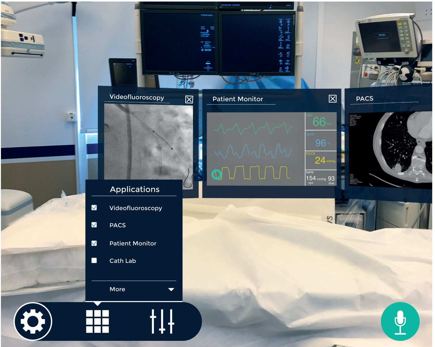
Fig 34: The augmented reality system from the cardiologist's point of view. The "Settings" panel and the voice control icon are tag-along elements, the applications in the background are fixed elements, fixed to a position in the room.
