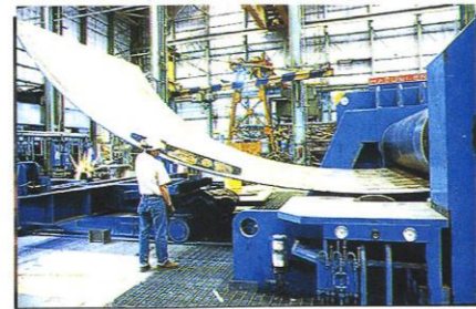
Steel bending. Workers program the desired shape into a robotic bending machine, which shapes the metal using 1000 tonnes of pressure.
