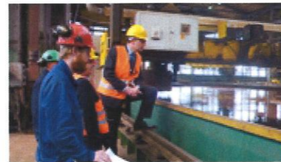
Steel cutting marks the production start of a shipbuilding project. The plates are cut in large basins. Water reduces the toxic emissions produced by the cutting laser.
