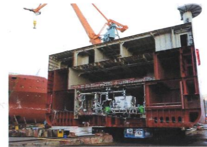
The hull is welded in blocks, instead of in one whole piece for easier installation of fittings and wires.
