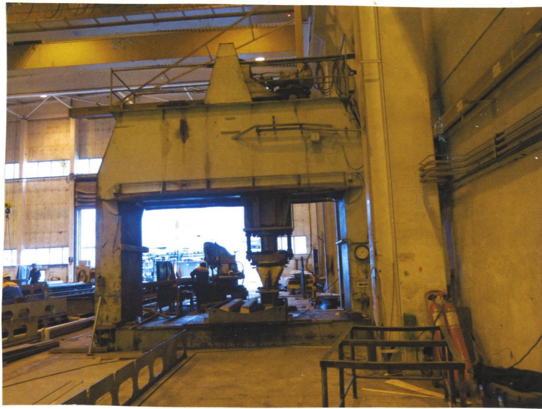
THE HYDRAULIC PRESS FOR CURVING THE STEEL PLATES
