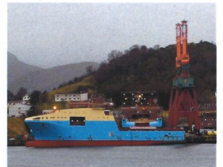
"outfitting", is the process in shipbuilding that follows the float-out of a vessel. All the remaining construction of the ship is completed and readied for delivery to her owners. Since most of the fitting-out process is interior work, this stage can overlap with latter stages, such as the sea trials.
