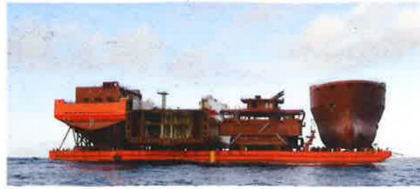
The ship is built in sections. The material is steel.
