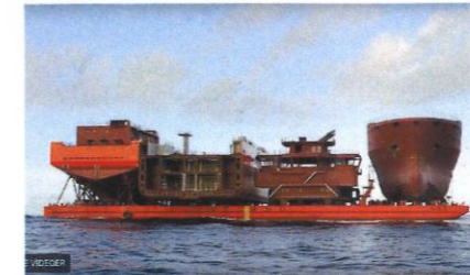
The hull is welded in blocks, instead of in one whole piece for easier installation of fittings and wires.
