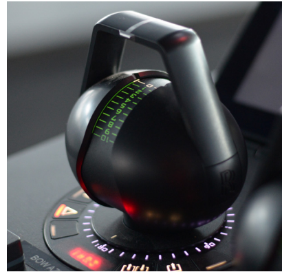
2x azipod thruster controllers 1 for portside 1 for Starboard
