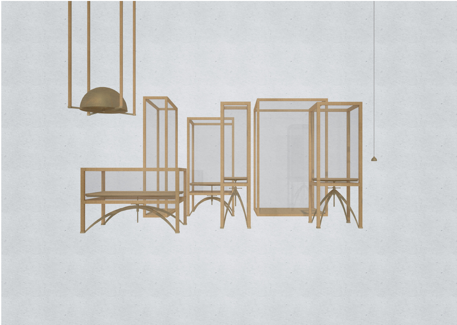
Family of vitrines From left to right: Sound shower, Adjustable table vitrin, Tall narrow vitrine for hanging objects, Large adjustable cabinet vitrine, Slim, adjustable cabinet vitrine, extra large vitrine for floor standing objects, Medium adjustable cabinet vitrine, Hanging mono hand-size loudspeaker.
