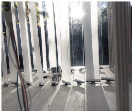
Testing the model for light analysis and Arduino data collection. Both wind and light data were collected and analyzed through 5 light sensors and 2 wind sensor placed in exterior, interior, and the transition space.
