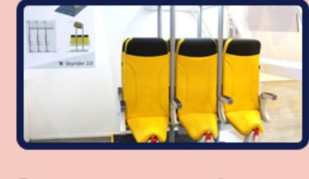
seats The vertical seat (standing seat, stand-up seat) is an airline seat configuration involves standing passengers travelling while being braced in position.
