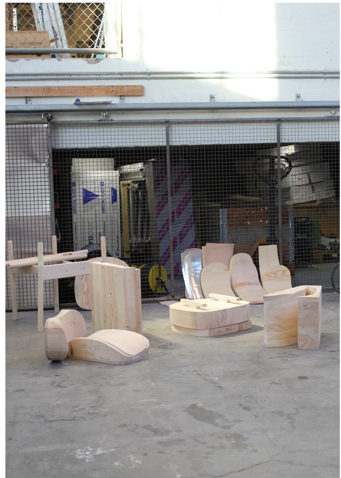
- Picture of the many molds and shapes from the process of creating the laminated seat and back.
