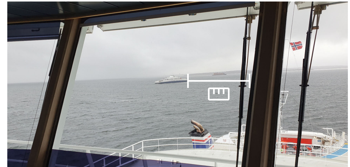
Measuring using window frame
