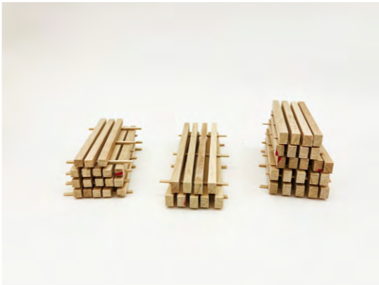
32 x 140x300 glulam beams 18 x 140x135 columns
