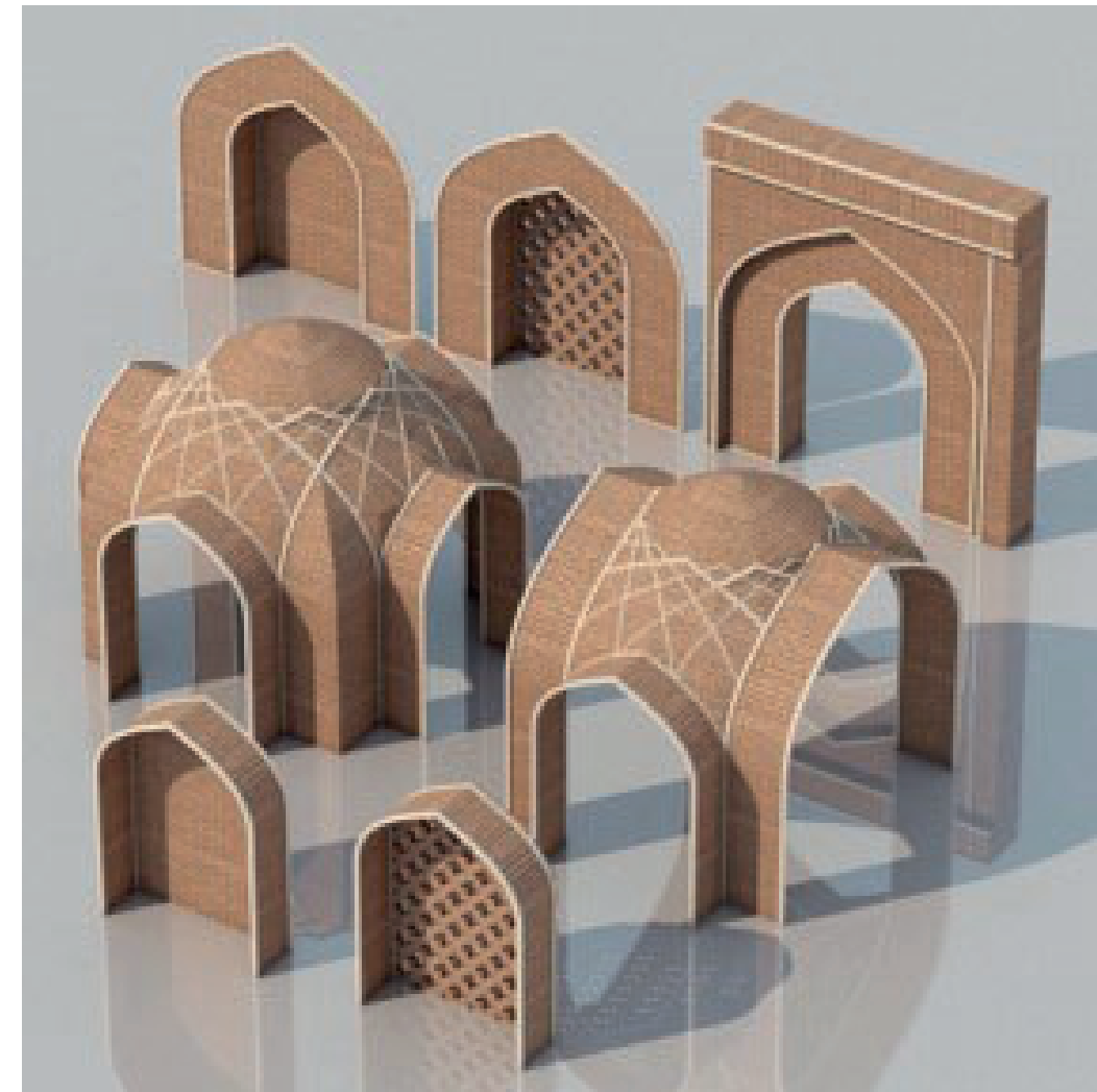
Geometric design of a masonry lattice space dome tittles Karbandi in Persian architecture
