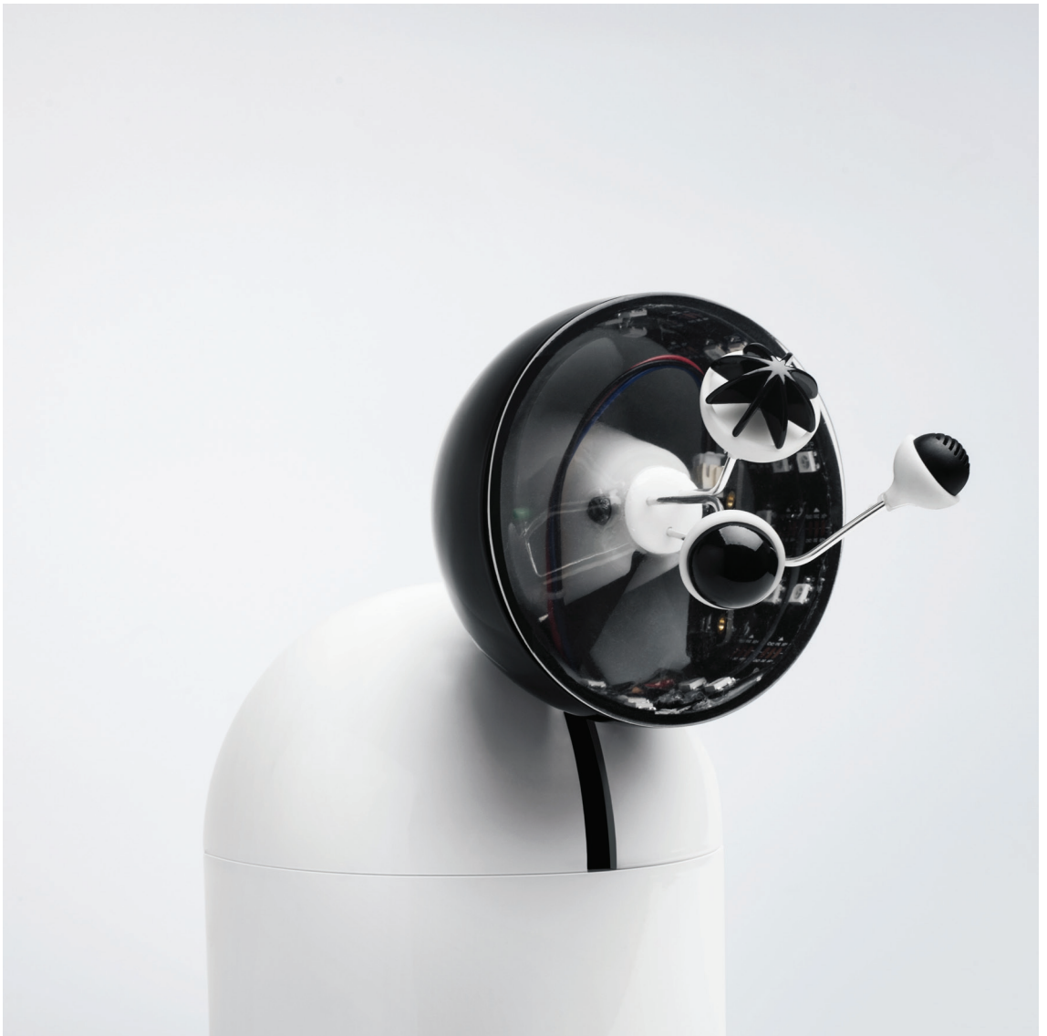
Figure 1.9 A functioning LO prototype showing the structure of the base and adjustable head with vision sensor and LED light (Zou, 2020).
