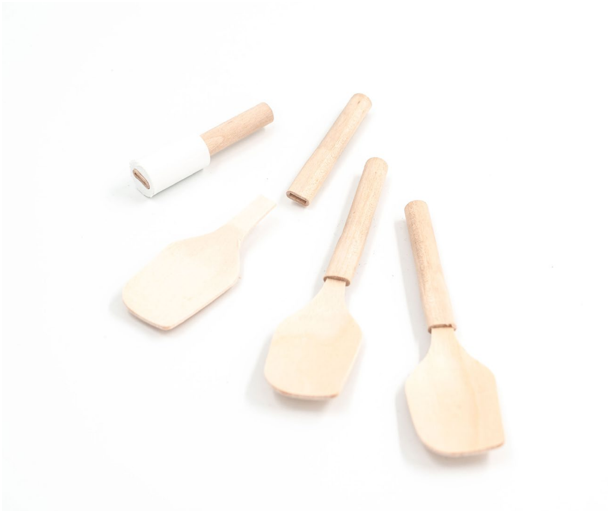
Two-part spoons with one-part mould for forming joint feature on the handle part.
