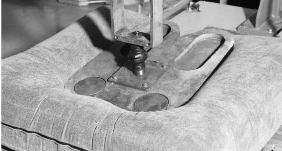
This photo shows the machine that does the test: 2. INDENTATION FORCE DEFLECTION (IFD) (20)
