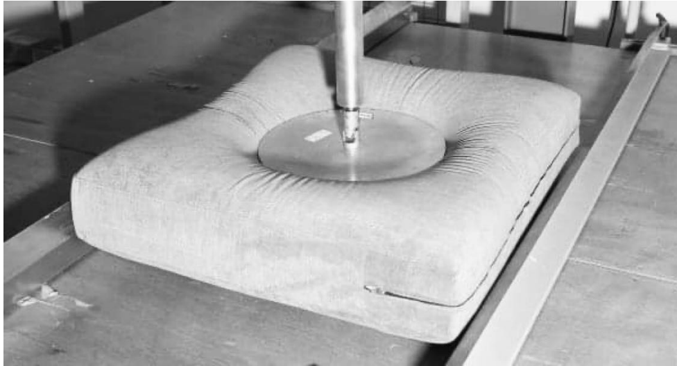
This photo shows the machine that does the test: 1. INDENTATION LOAD DEFLECTION (ILD) (20)
