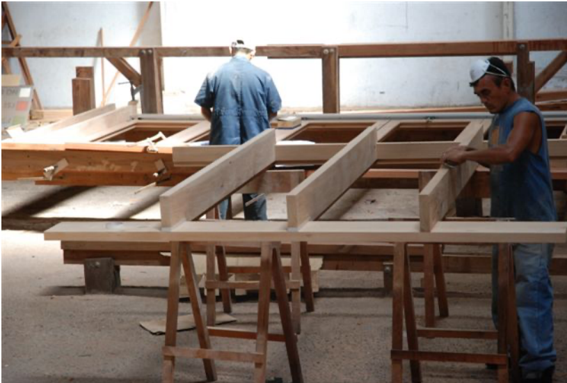
Figure 3. Hardwood joinery, fabricated in a workshop in Nicaragua, for site assembly. Strange House, London, Hugh Strange Architects. 2010. (Photo: Matthew Falkiner)
