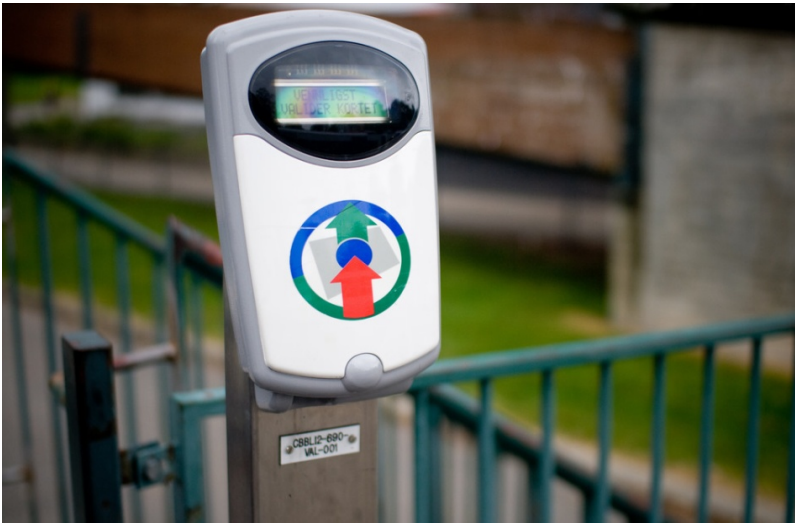
Figure 1.1. Oslo is currently introducing an RFID-driven electronic ticketing system for public transportation. The image shows an RFID card reader at a subway station (2010).
