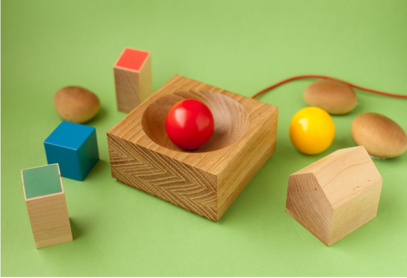
Figure 2.3. 'Bowl' was a video player driven by an embedded RFID reader in a wooden bowl. By placing various RFID-embedded objects in the bowl, video streams could be controlled on a connected TV set (Martinussen et al., 2007).
