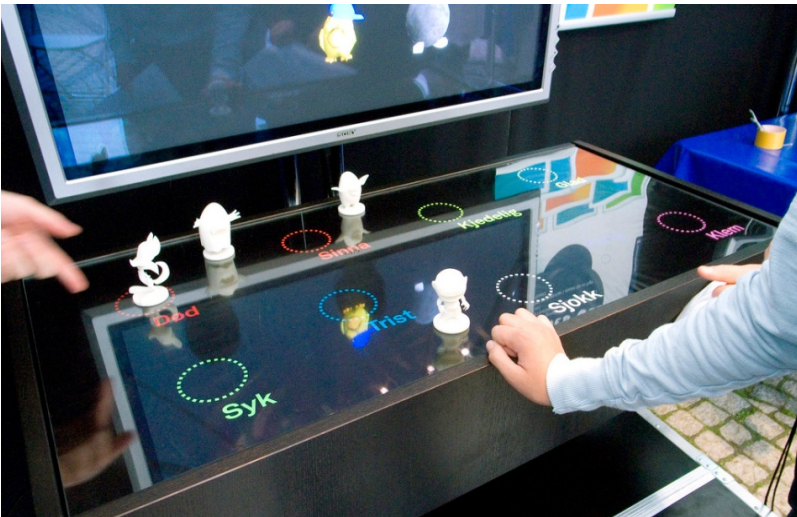
Figure 3.4. Orooni table: An RFID reader is mounted under each of the 10 circles in the table. Moving a character over the circle would trigger a continuous animated event on the screen.
