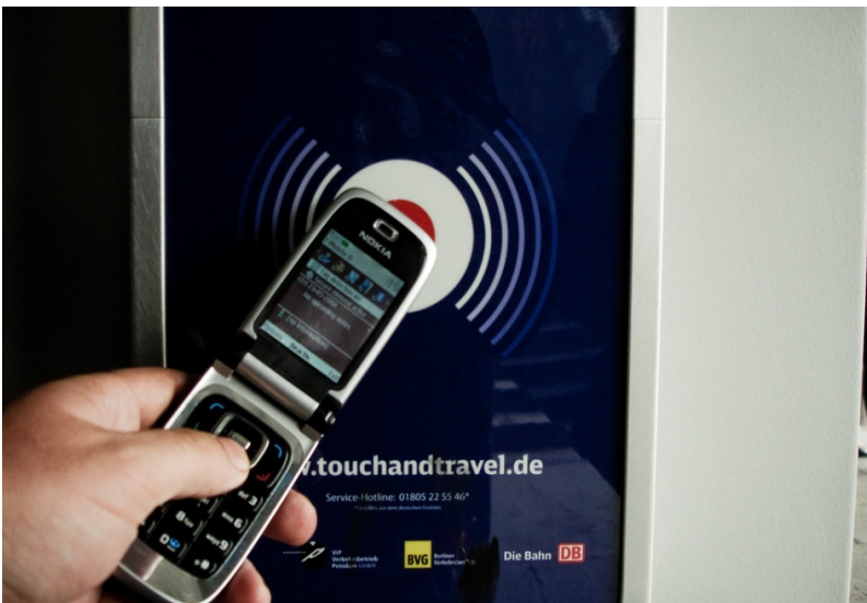
Figure 2.9. A smart poster equipped with an RFID tag may be read by an RFID-enabled phone.
