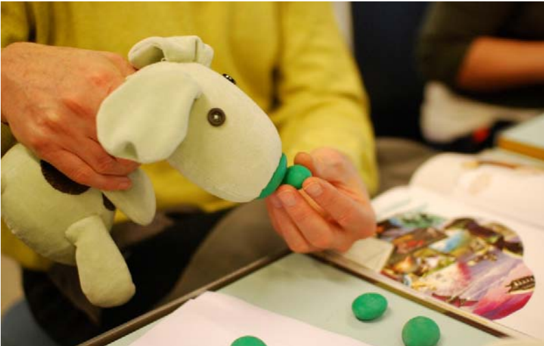
Figure 2.4. 'Sniff' allowed blind children to trigger various behaviours in a toy by 'sniffing' RFID-embedded objects (Johansson, 2009).
