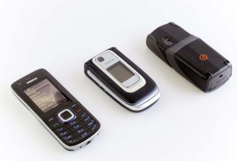
Figure 2.8. Nokia has been pioneering the marketing of RFID-enabled mobiles in the West. Shown are three RFID-equipped Nokia handsets that have been used in the Touch project (from top right, the 5140i, the 6131 and the 6212).
