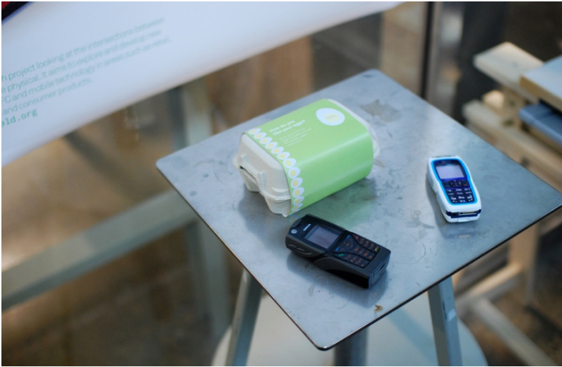
Figure 3.5. The egg carton allows access to a timer application when the phone hovers over it.
