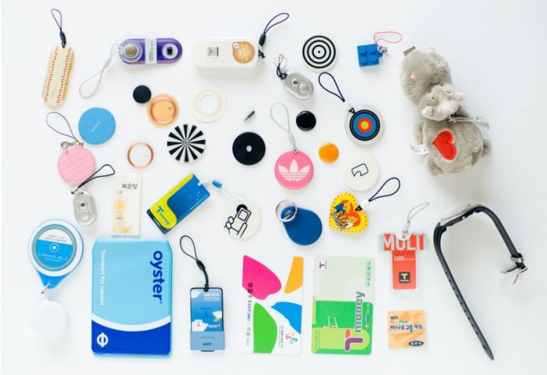
Figure 2.7. RFID tags may be embedded in all kinds of objects. The image shows a small part of the (passive) RFID tag collection from the Touch project.
