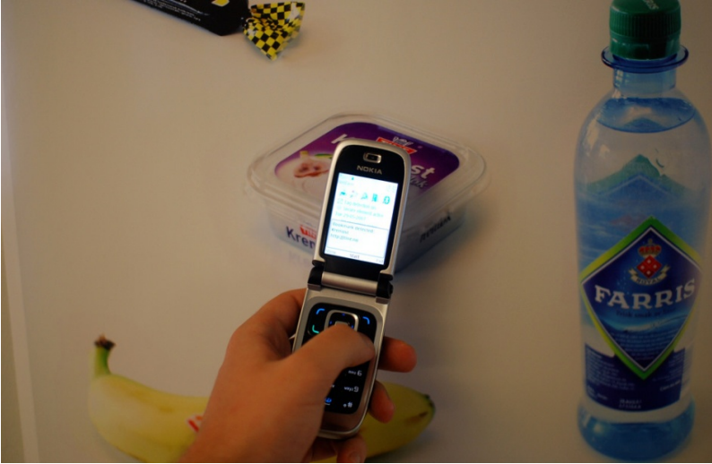
Figure 3.2. The Touch project created a small demo of a smart poster using the inbuilt functionality of the NFC phone. Although simple, it provides hands-on experience of the current offerings in RFID-driven phone interactions.
