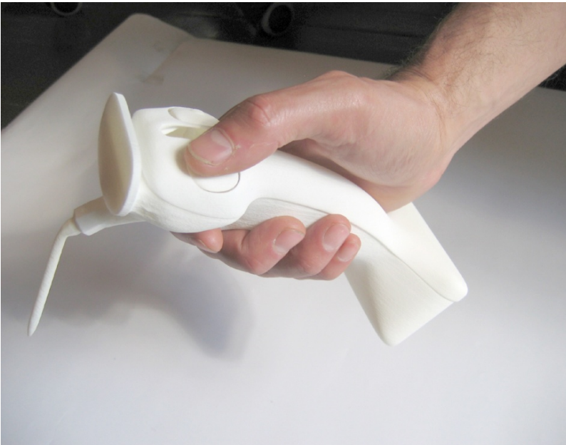
Figure 2.10. A prototype of an interface offering tangible interactions for programming robots created by the author for ABB research.
