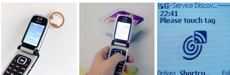
Figure 1. Aspects of NFC interaction using inbuilt software on the Nokia 6131 NFC phone. The image on the left shows a simple transfer of a hyperlink from a tag. The centre image shows the same functionality in relation to an interactive poster. The image to the right shows the inbuilt interface on the Nokia phone.
