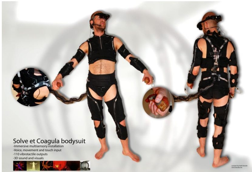
Figure 4-28 The SeC bodysuit. The up to 120 effectors are equally distributed throughout the suit, effectively covering the whole body. The user holds the pressure sensitive devices in each hand.
