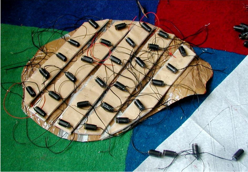
Figure 6-12 Showing the density of the effectors on one of the leg pads. Effectors are being mounted on top of the sensors (here bundled into what is seen as five stripes), facing inwards to the body.
