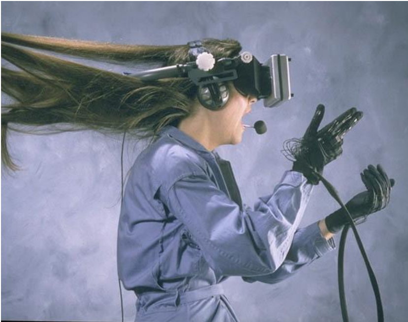
Figure 4-6 The NASA HMD by Scott Fisher, the so called VIEW (Virtual Interface Environmental Workstation). Image courtesy of Scott Fisher, NASA-Ames Research Center.
