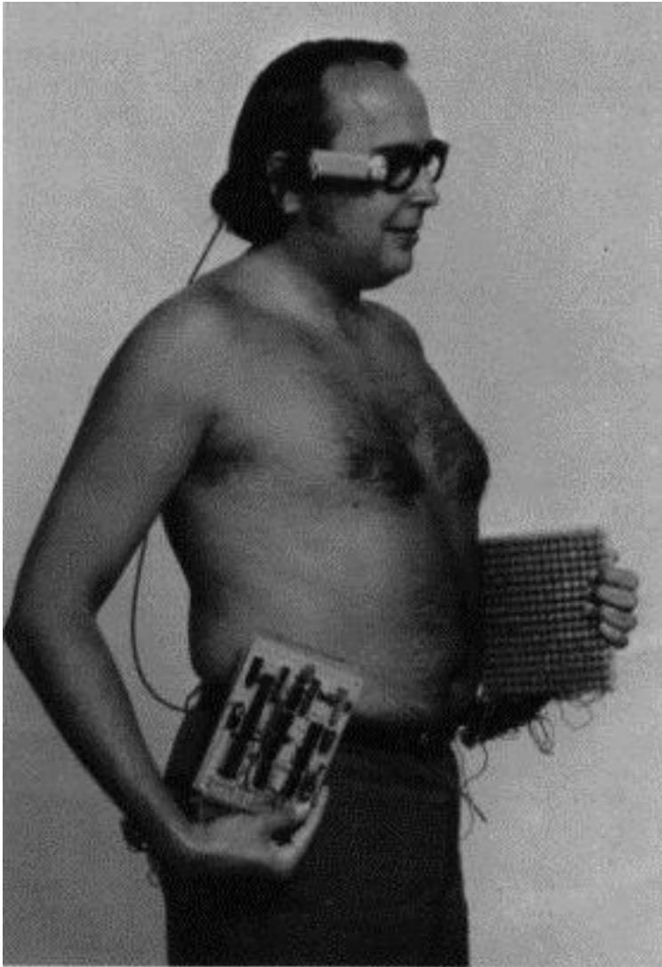
Figure 4-11 Portable sensory substitution system developed by Paul Bach-y-Rita and colleagues (1969). © Paul Bach-y-Rita.
