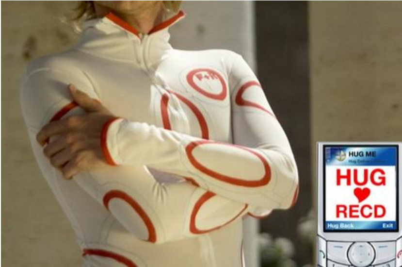
Figure 4-21 The Hug Shirt. Areas with sensors marked with orange circles. © CuteCircuit.
